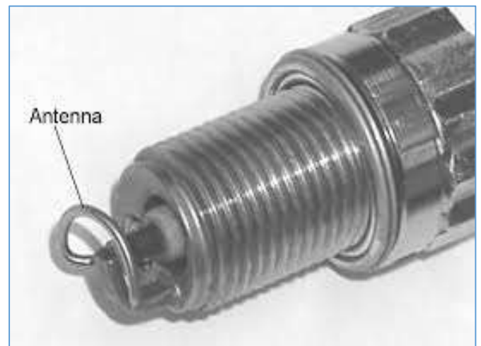
Figure 6 Microwave Assisted Ignition System (7)
