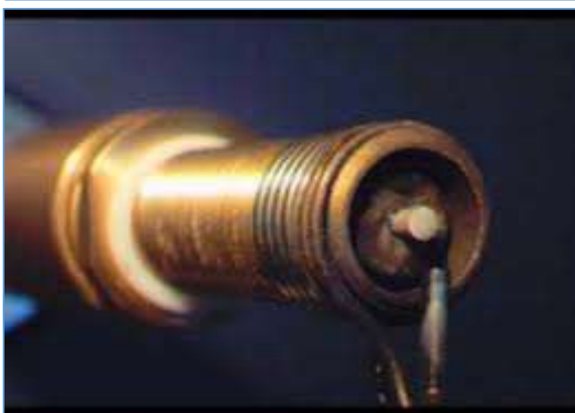
Figure 9 Radio Frequency Spark Ignition (RFSI)(12)
