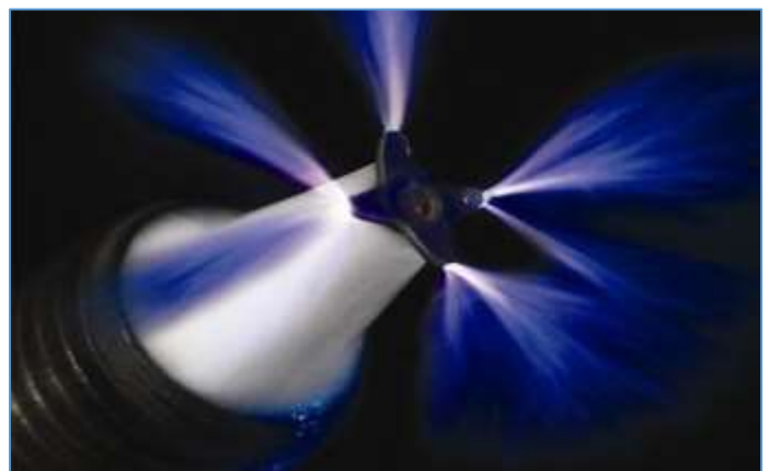
Figure 8 Corona Discharge Ignition System(11)
