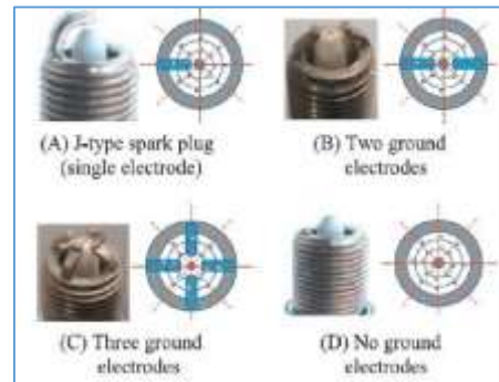
Figure 4 Ignition System without Ground Electrodes(5)
