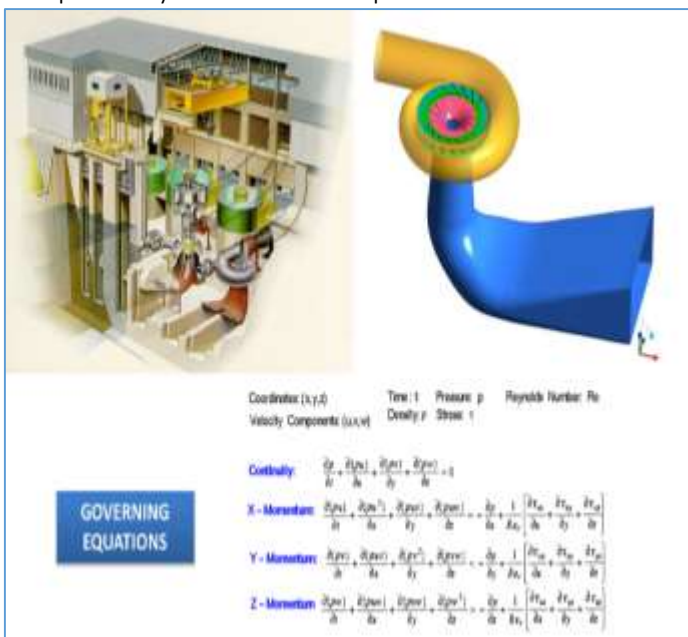
Figure 4: Numerical simulation of reaction turbine and Governing Equations :
